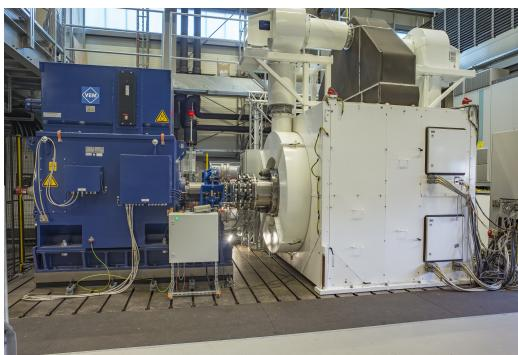
**Abb. 27:** Generator Converter Laboratory GeCoLab
